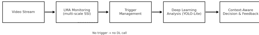
Fig. 1. System Architecture Diagram showing the integration of LMA monitoring with deep learning analysis
